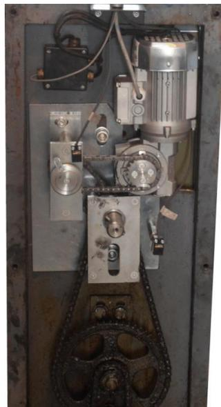
**2:3 Inside Wheel Box Fitted with an Electric Winder**
