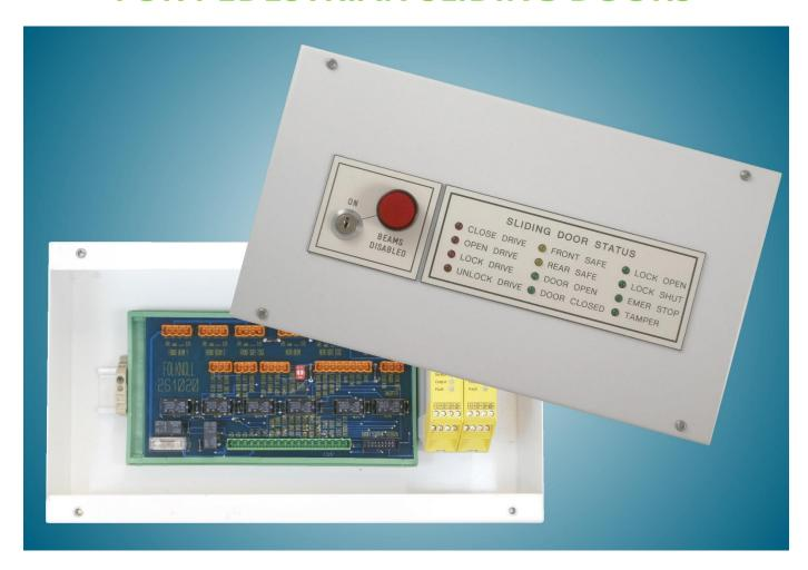
Cable terminal box for security system multi-core cable with interface for Portable Engineer's Terminal
