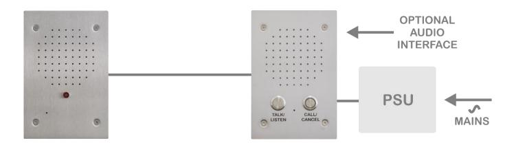
1-off 970.56 vandal resistant passive outstation 1-off 970.50 vandal resistant master station Optional 970.59 audio interface 1-off 970.00 system PSU
