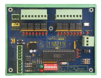
RS485 16-ZONE OUTPUT CONTROLLER Can mimic RS485 alarms from 16-zone input controller Can mimic alarms from 3 x 5-zone strip alarm controller Consolidated alarm and fault management function Output for auxiliary beacon / sounder Compatible with Folknoll RS485 networking systems Compatible with Folknoll SNI IP networking
