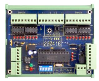
RS-485 16-ZONE INPUT CONTROLLER Accepts 16 alarm zones or 8 alarm zones with faults Diagnostic LEDs for maintenance Alarm accept output Fault signal monitoring mode Compatible with Folknoll RS-485 networking systems Compatible with Folknoll SNI IP networking
