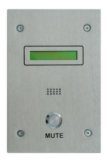
ALARM INDICATOR PANEL FOR UP TO 8 ALARMS BS 8300-9 compliant Alerts staff to system alarms and faults 16-character LCD display Mute button Integral sounder Output for auxiliary beacons / sounders Vandal resistant, stainless steel, construction Flush or surface mount, anti-tamper fixings available Suitable for use in public areas
