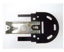
The base end cap plate is first held in position on to the architrave back box through either of the slots in the plate. One slot allows longitudinal movement the other horizontal if fitting to paired box ends. As above, once the end cap plate is held in position on the architrave box the wall can be marked for drilling. Remove plate to enable drilling and plugging. Proceed with the wiring and cover plate fitting as in No1
