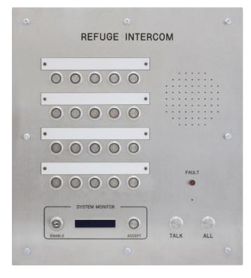
STANDARD SYSTEM MASTER FOR UP TO 20 OUTSTATIONS LCD status display, speaker, microphone, fault LED High audio output for noisy environments (max 80dB) Tough vandal resistant construction Stainless steel faceplate Keyed enable switch, vandal resistant buttons Custom labels available Anti-tamper fixings available Ideal for public spaces
