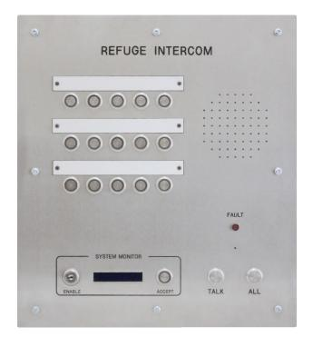
STANDARD SYSTEM MASTER FOR UP TO 15 OUTSTATIONS LCD status display, speaker, microphone, fault LED High audio output for noisy environments (max 80dB) Tough vandal resistant construction Stainless steel faceplate Keyed enable switch, vandal resistant buttons Custom labels available Anti-tamper fixings available Ideal for public spaces
