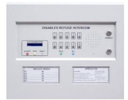
MASTER STATION AND CONTROL SYSTEM FOR UP TO 10 OUTSTATIONS Keyed enable switch LCD status display and Fault LED Internal speaker, internal microphone High audio output for noisy environments (max 80dB) Audio path testing, internal and external triggers Mains supply monitoring and reporting I/O for BMS or other external systems Matches standard fire panel size and quality Custom labels Surface or semi flush mount, Security fixings
