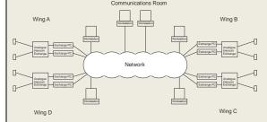
Local Videcom Systems can be networked over IP to form site-wide intercom systems. Video and audio can be streamed across the network allowing authorised operators to handle calls from intercom users from across the site.
