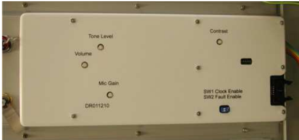
Fig 11:15 Rear Panel of Compact Master Station Door
